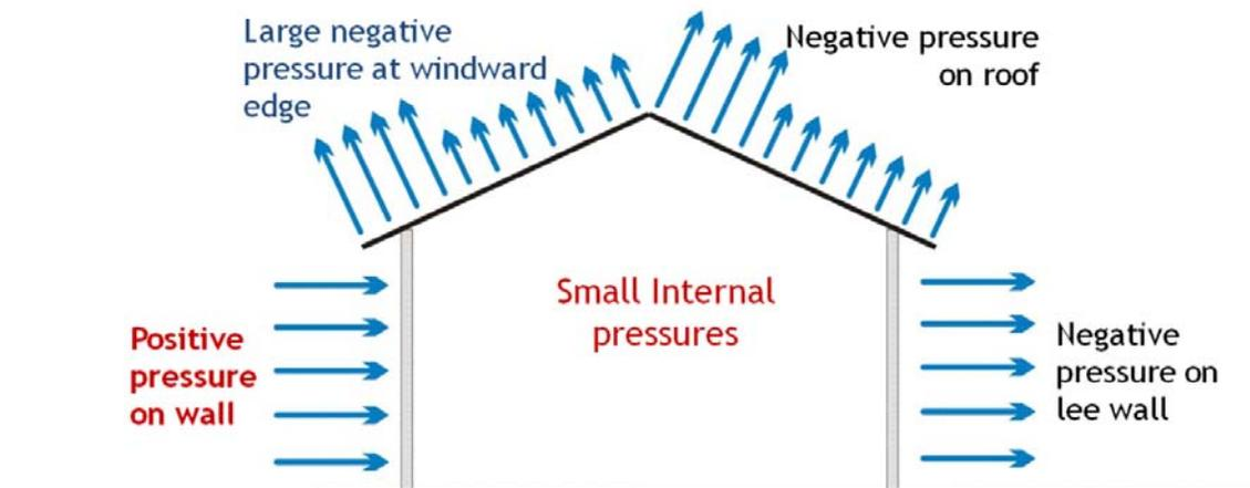
Figure 3 Representation of wind forces on a house
