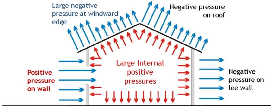
Figure 4 Wind forces with a dominant opening in windward wall
