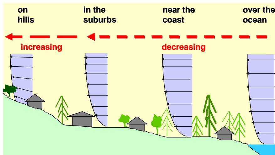
Figure 2 Representation of wind speed slowing for rough terrain and then increasing for the topographic slope
